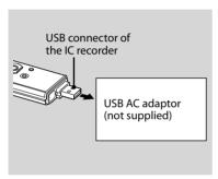
You can charge the rechargeable battery by connecting the IC recorder to an AC outlet using a USB AC adaptor AC-U50AV AC-U50AD (not supplied).
